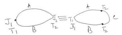
→ This law states that if a 3<sup>rd</sup> metal 'C' is inserted between A and B at either junction. And the new junction AC or BC at the same temperature (T<sub>1</sub> or T<sub>2</sub>), then the emf is unchanged.
