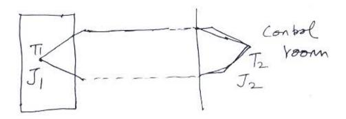
→The extra leads used for lead compensation may be of same material of thermocouple or, of different material having the same thermal conducting properties of the metal used.
