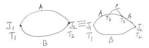
→This law states that if a 3<sup>rd</sup> metal is introduced into A (or B) and the two new junctions are at same temperature T<sub>3</sub>, then emf of the thermocouple is unchanged.
