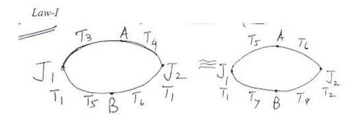
→ It states that the emf of a given thermocouple depends only on the temperature of the junction and independent of the wire connecting the junction.
